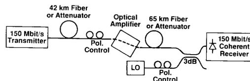
Fig. 1. Coherent transmission setup with optical amplifier.
