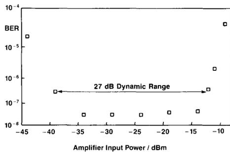
Fig. 2. Bit error ratio BER versus amplifier input fiber power  $P_{in}$  with constant total attenuation.
