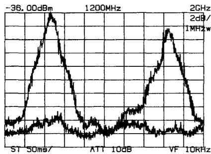
Fig. 15. IF spectra for two different polarization conditions.
