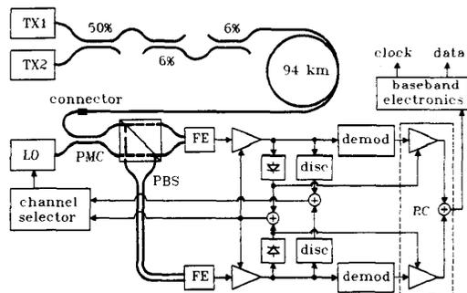
Fig. 9. Experimental setup for polarization diversity: PMC = polarization-maintaining coupler, PBS = polarization beam splitter, FE = front end, demod = demodulator, RC = ratio combiner.
