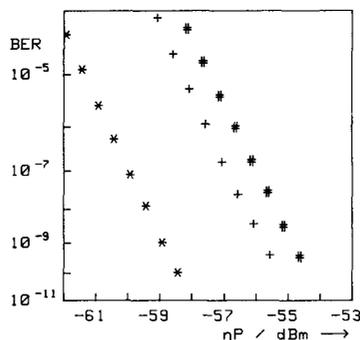
Fig. 17. Bit error ratios versus received power  $\eta P$ : (\*) standard heterodyne, (+) best and (#) worst cases of active, data-synchronous polarization switching.
