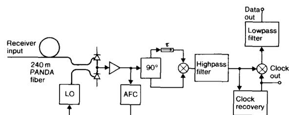
Fig. 14. Experimental setup for data-induced polarization switching in the receiver.
