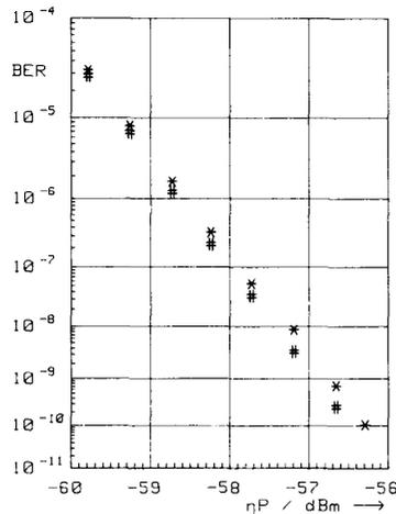
Fig. 7. Bit error ratio for receiver with endless polarization control against received power  $\eta P$  for  $2^{15} - 1$  (\*) and 1010 (#) data patterns.
