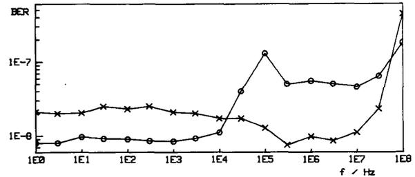
Fig. 13. Bit error ratio versus polarization modulation frequency for polarization diversity ( $\circ$ ) and data-induced polarization switching ( $\times$ ).
