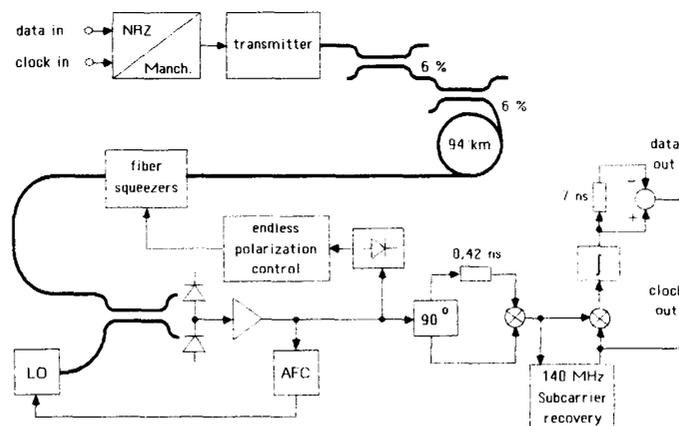
Fig. 5. FSK heterodyne system with Manchester coding and endless polarization control.
