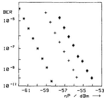
Fig. 16. Bit error ratios versus received power  $\eta P$ : (\*) standard heterodyne, (+) best and (#) worst cases of data-induced polarization switching.
