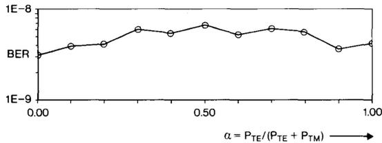
Fig. 12. Bit error ratio versus signal polarization for polarization diversity.
