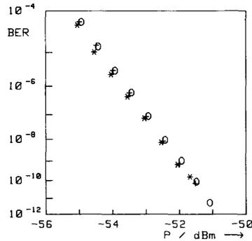
Fig. 11. Bit error ratio versus power at input connector of polarization diversity receiver ( $\alpha = P_{TE}/(P_{TE} + P_{TM})$ ;  $\alpha = 0 \leftrightarrow *$ ;  $\alpha = 0.5 \leftrightarrow \circ$ ;  $\alpha = 1 \leftrightarrow +$ ).
