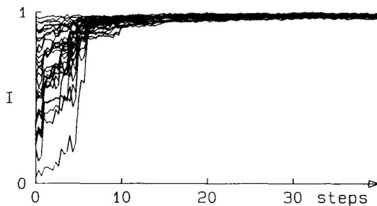
Fig. 8. Measured transient responses of endless polarization control system from random starting points; IF intensity  $I$  versus number of maximization steps.
