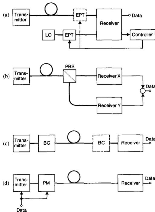
Fig. 1. Coherent transmission system using (a) polarization control, (b) polarization diversity, (c) data-induced polarization switching, (d) active, data-synchronous polarization switching. EPT = endless polarization transformer, PBS = polarization beam splitter, BC = birefringent component, PM = polarization modulator. Dashed lines specify alternative component placements.
