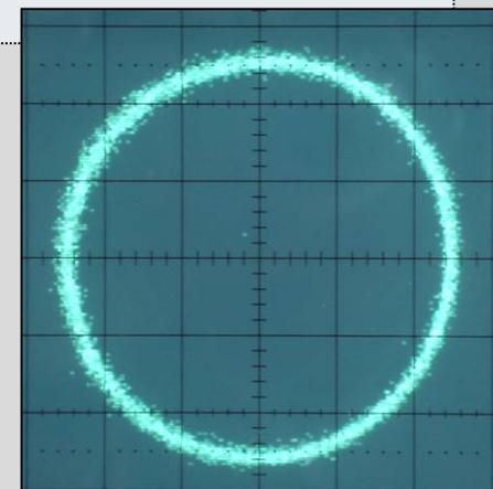
**Automatic frequency control & carrier recovery needed!**
