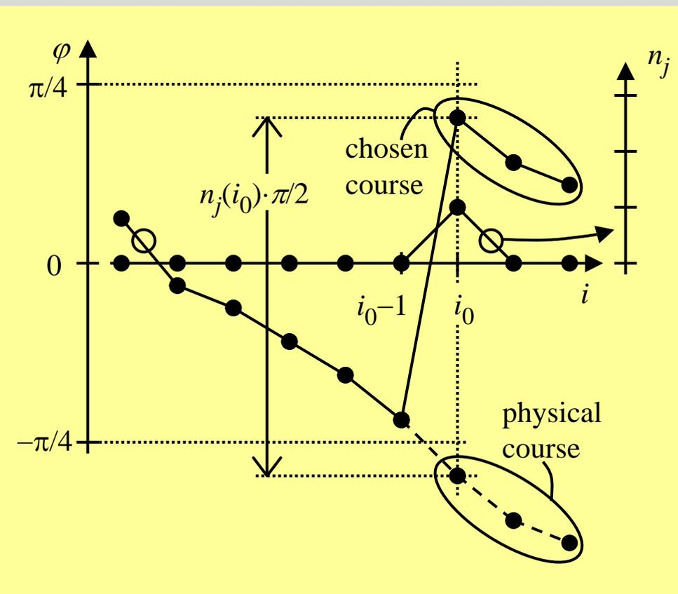
*Inconsistency between estimated IF phase and (most likely) physical course is detected and encoded for differential decoding as a quadrant jump number  $n_j$*
