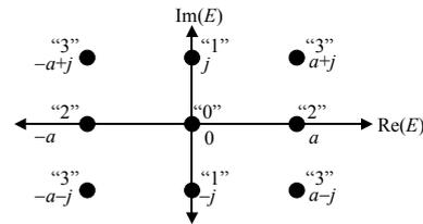
Fig. 2: Electrical field modulation constellation ( $a = \sqrt{2}$ ). A quaternary intensity modulation results.
