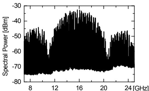
Fig. 5: Heterodyned electrical spectrum of the 2x10Gbit/s 9-QAM = 4-IM signal (RB: 100KHz)
