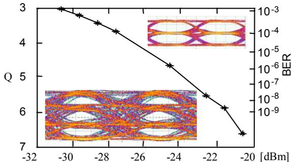
Fig. 4: Back-to-back receiver sensitivity and corresponding eye diagram for 2x10Gbit/s QAM signal (inset: electrical duobinary eye diagram (top)).
