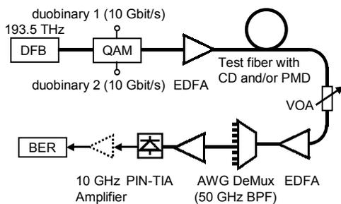
Fig. 3: 20 Gbit/s 9-QAM (4-IM) transmission setup
