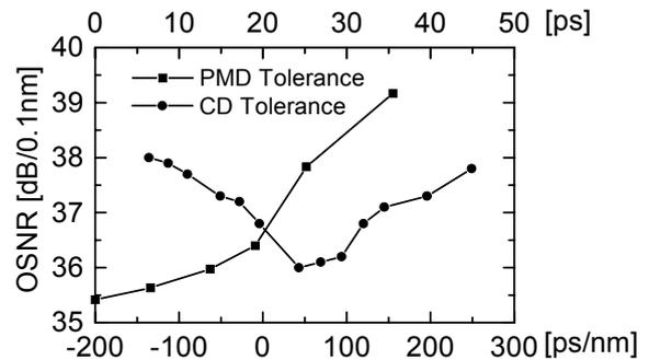
Fig. 6 OSNR needed for a BER of  $10^{-9}$  versus CD in ps/nm and PMD in ps.
