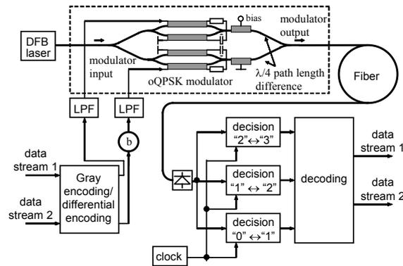
Fig. 1: Schematic of the optical 9-QAM modulation using duobinary low pass filtering (LPF) at the transmitter and the 4-IM receiver
