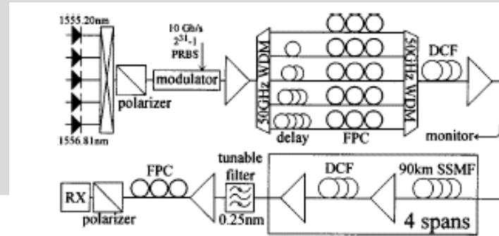
Fig. 2. Schematic of the transmission line setup. (FPC-fiber polarization controller; RX-receiver; SSMF-standard single-mode fiber).
