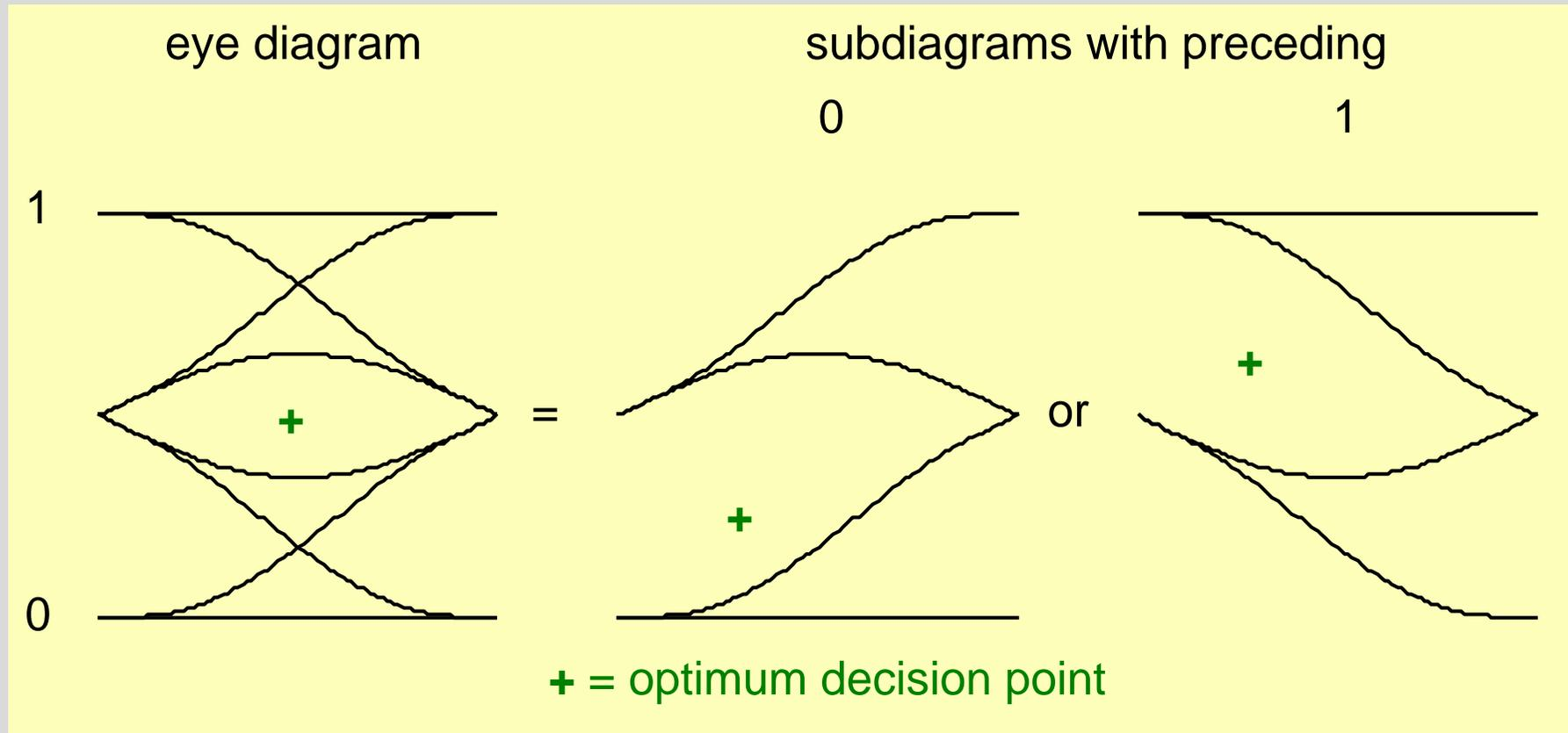
Due to negative binomial or  $\chi^2$  noise from optical amplifiers, system penalty is larger than subdiagram opening penalty.
