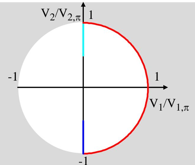
For circular input polarization the output polarization is obtained by an azimuthal equidistant projection onto Poincaré sphere:
