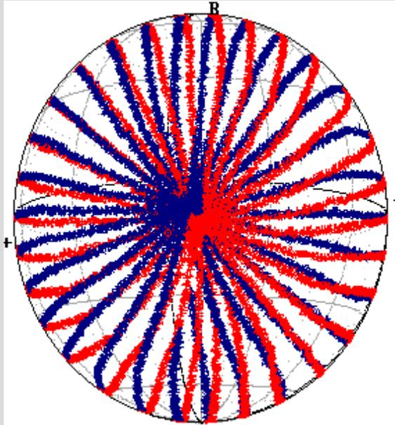
Continuous, endless polarization tracking on the 30 most critical great circles of the Poincaré sphere crossing the TE/TM “poles”. All other cases are better behaved.
