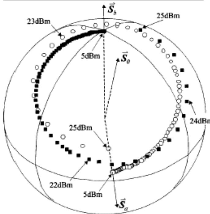
Fig. 1. Output Stokes vectors for the two signals. Labels show the launched peak powers of each signal. Between points, the power is changed by 0.2 dBm.
