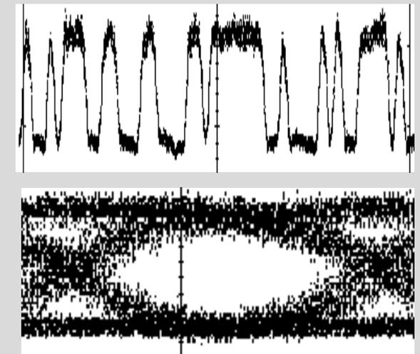
data output signal and its eye diagram
