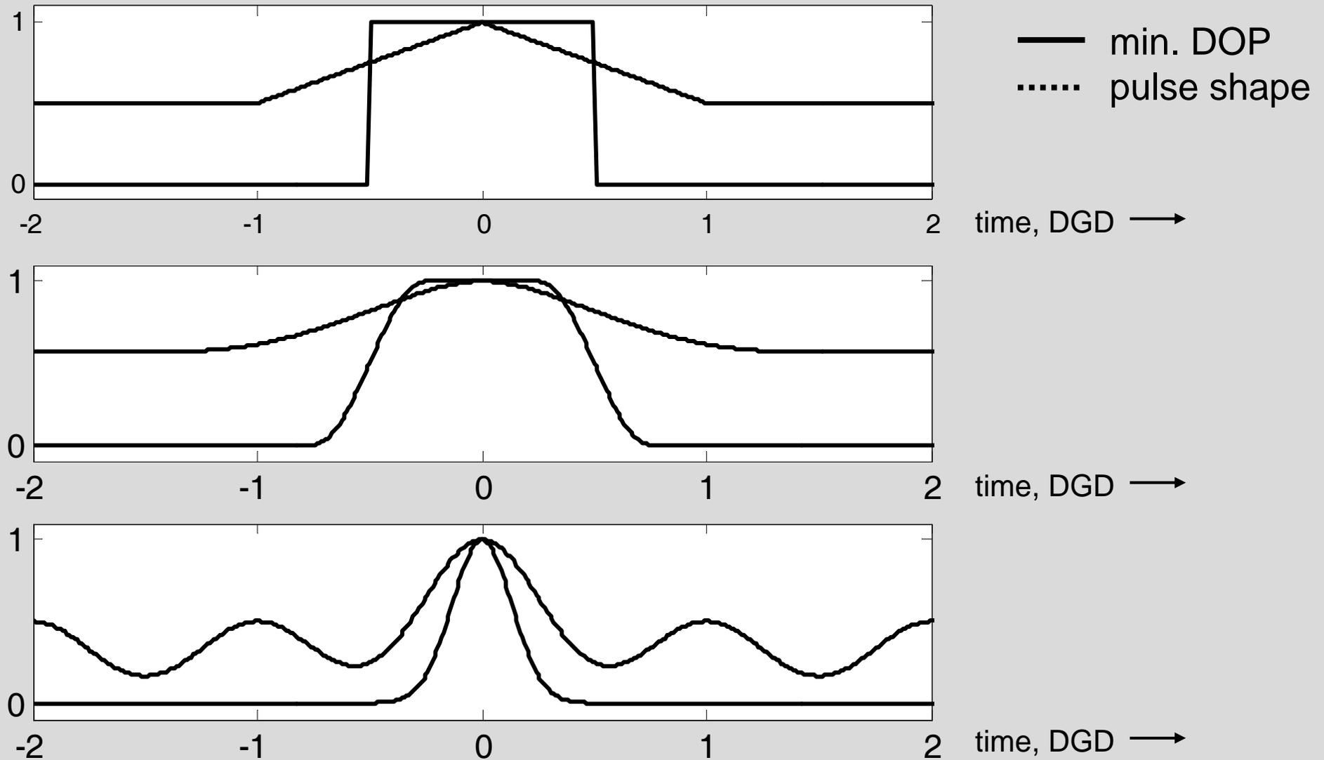
Readout is proportional to DGD, but only if pulses edges are shorter than DGD !
