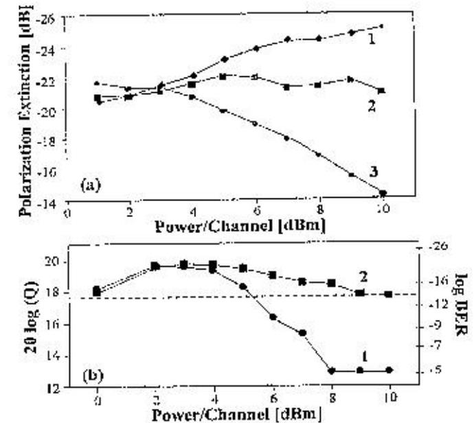
Fig. 4. (a) Maximum extinction possible by the polarizer versus launched power per channel for 1) a single modulated channel, 2) all channels unmodulated and 3) all channels modulated. (b) Measured  $Q$  factors versus launched power per channel both 1) with and 2) without the polarizer in front of the receiver.
