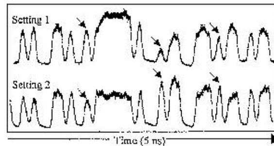
Fig. 3. Received bit patterns with the polarizer in front of the receiver for two different settings of the polarization controller. Arrows indicate large amplitude variations of the same bit.
