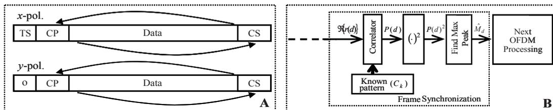
Fig. 1. A: Proposed OFDM frame in simulation for two polarizations (x-pol and y-pol)
