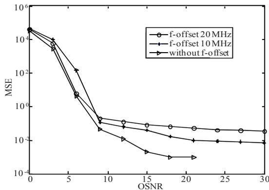
Fig. 3 MSE errors of OFDM frame
