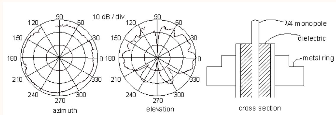
Fig. 5: Radiation pattern of a simple monopole antenna
