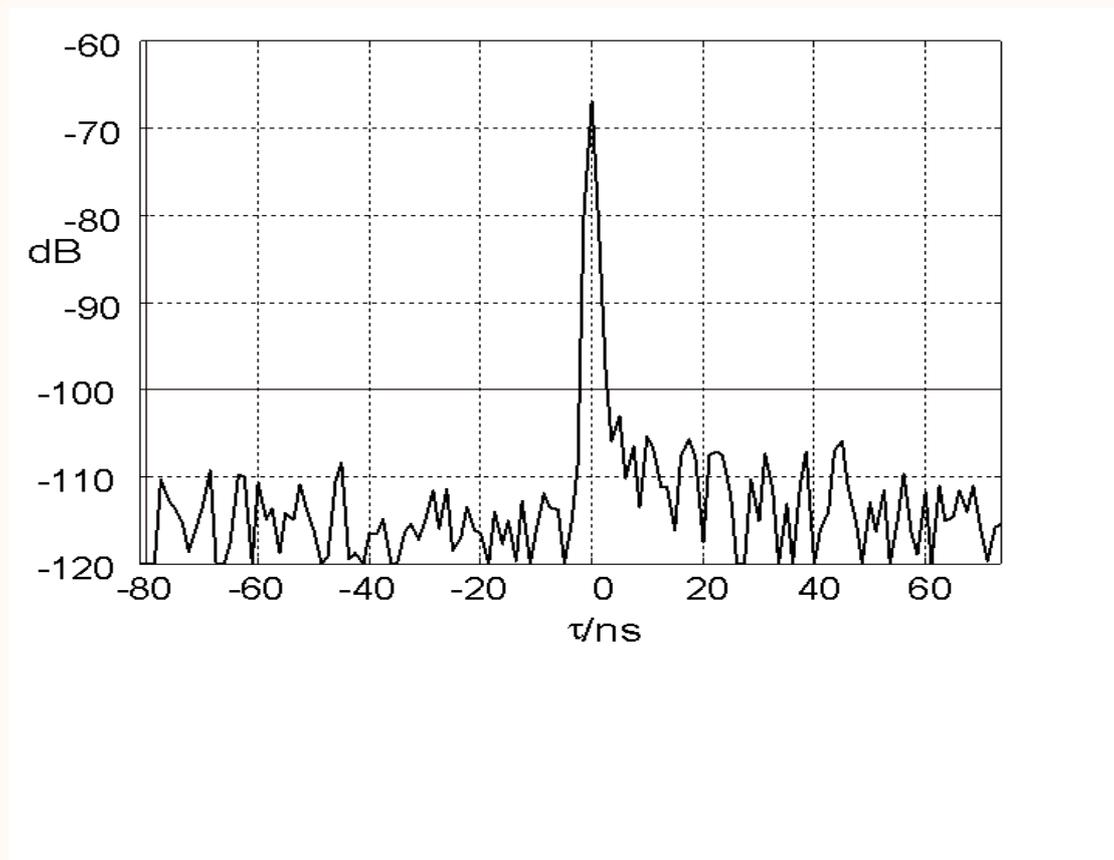
Fig. 2: Measured impulse response of a reference channel without multipath propagation.
