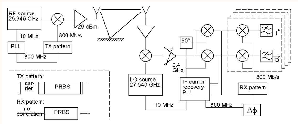
Fig. 1: Channel sounder block diagram
