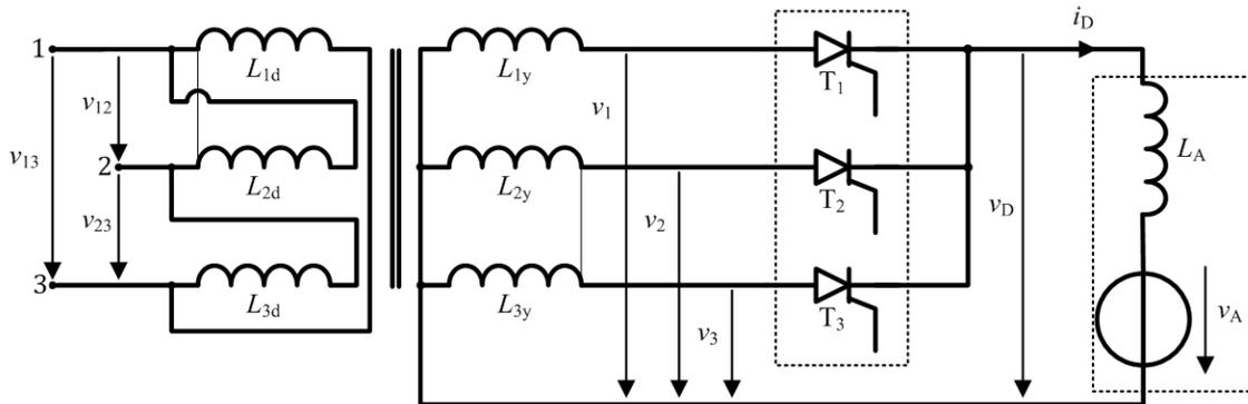
Figure 1: Three-phase half-wave controlled rectifier
