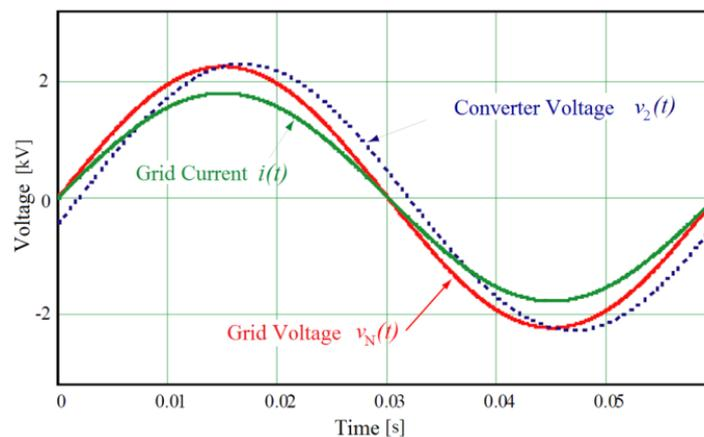
Figure 2: Voltages and currents transformed to the secondary side of the transformer
