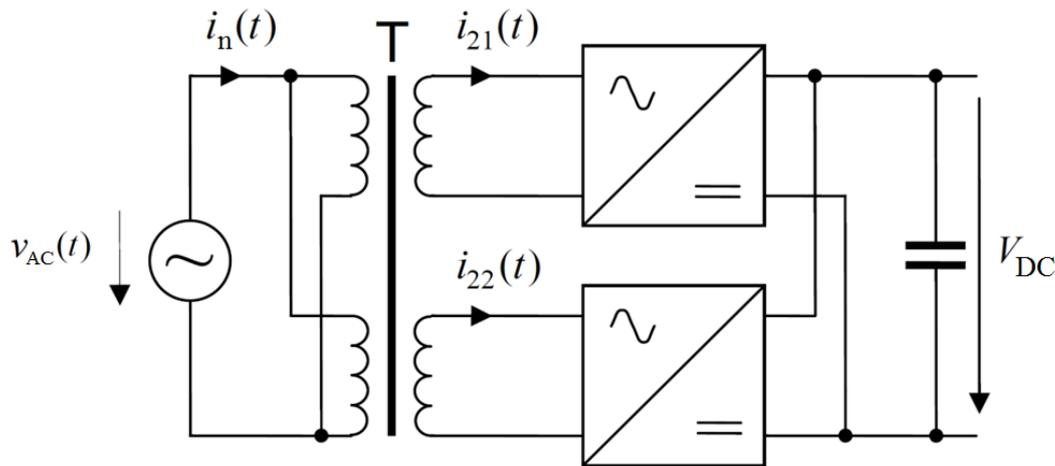
Figure 1: Power supply for a suburban train
