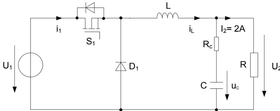
**Fig.1: Buck converter**
