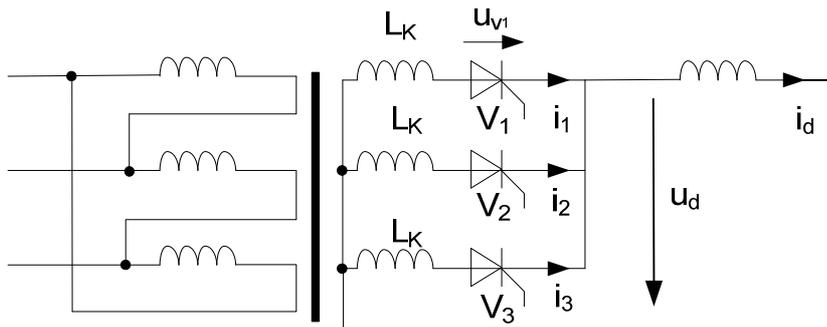
**Fig 4: Line commutated converter in M3 configuration**
