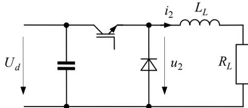
**Fig. 1** Buck converter with passive load
