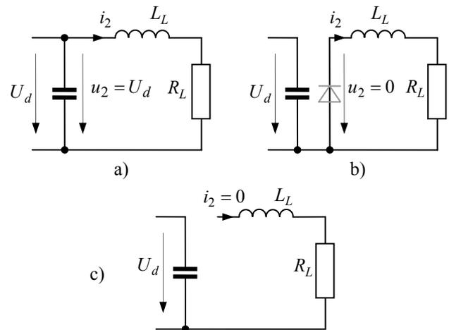
**Fig. 4** Equivalent circuits of buck converter
