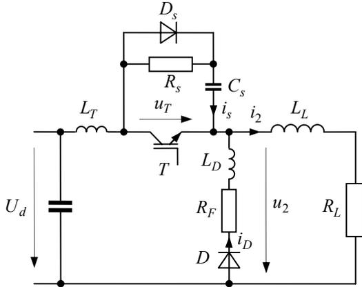
**Fig. 8** Buck converter with clamping circuit and parasitic elements
