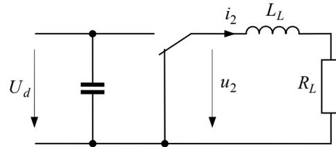
**Fig. 3** Equivalent circuit of buck converter used for investigation of basic behavior
