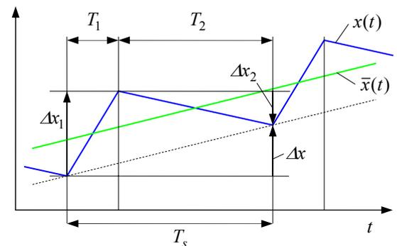
Fig. 5 State variable during a switching period
