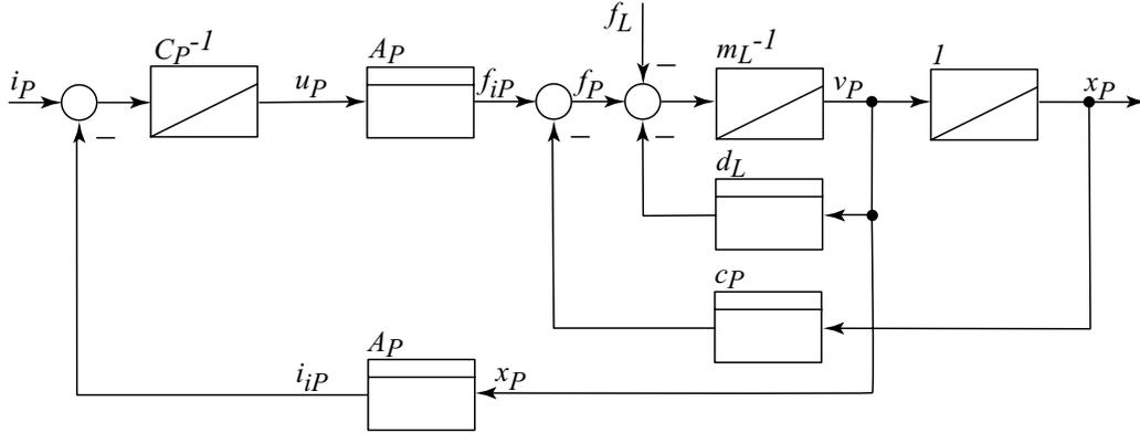
Fig. 3: Block diagram of piezoelectric actuator loaded by prestress spring and load mass
