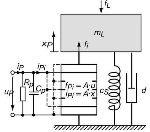
Fig. 2: Piezoelectric actuator loaded by prestress spring and load mass
