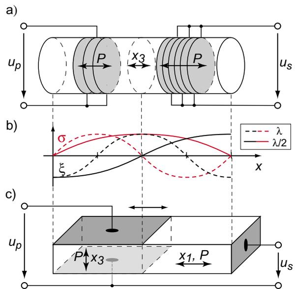
Fig. 9: Piezoelectric transformers
