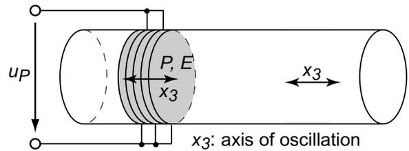
Fig. 8: Sonotrode with stack actuator making use of  $d_{33}$ -effect
