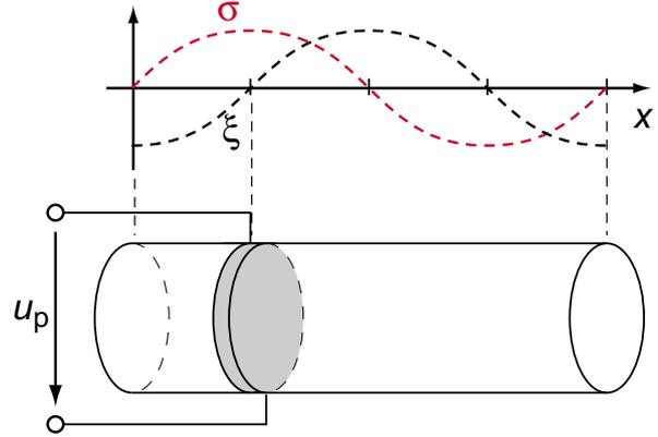
Fig. 6: Resonant operated sonotrode
