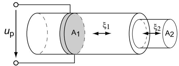
Fig. 7: Sonotrode with cross-sectional reduction
