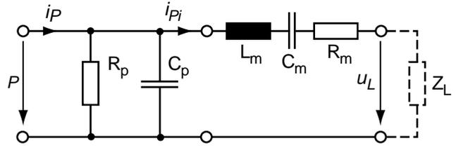
Fig. 4: Equivalent circuit of loaded piezoelectric actuator
