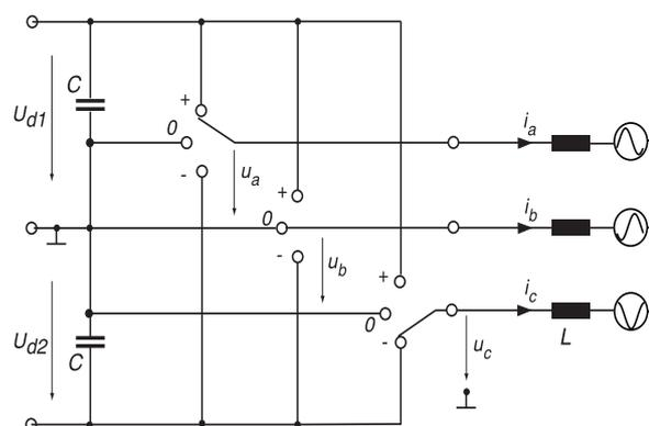
Fig. 2 Equivalent circuit of three-level converter
