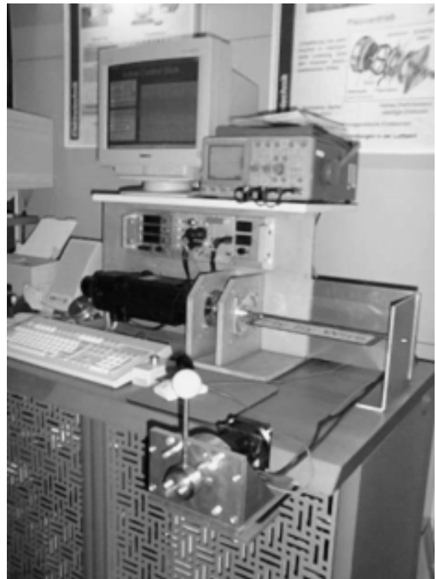
Figure 6. One axis prototype ACS driven by an USM exhibited and demonstrated on a fair in March 1999 in Paderborn, Germany. Since a DC-motor serves for simulating the rudder actuator active force feedback can be shown by this experimental assembly, too.
