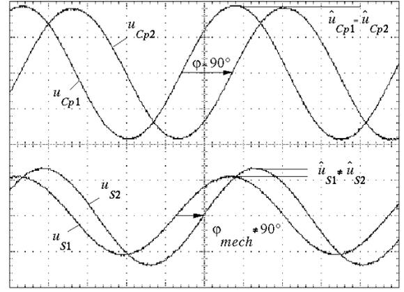
Figure 8: Measured phase voltages  $u_{Cp1}, u_{Cp2}$  and sensor signals  $u_{S1}, u_{S2}$  of USM in case of symmetrical feeding
