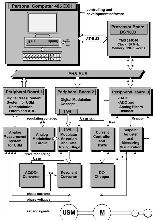
Figure 1: Experimental set-up for ultrasonic drives
