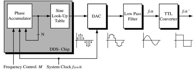
Figure 11: Direct Digital Synthesizer
