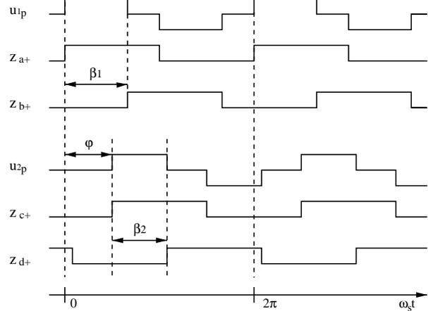
Figure 5: Inverter voltages in accordance with quantities  $f_s$ ,  $\phi$ ,  $\beta_1$ ,  $\beta_2$
