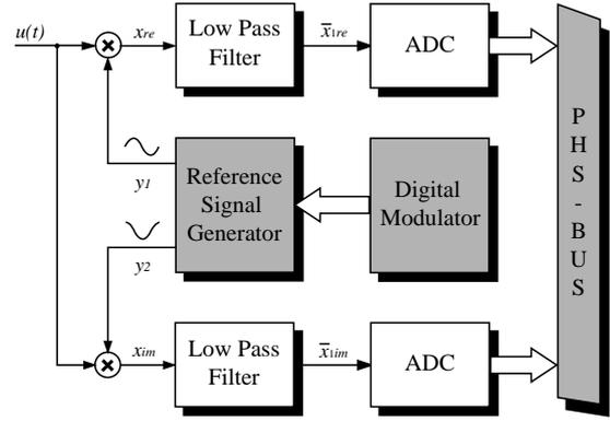
Figure 13: Measuring system by analog demodulation
