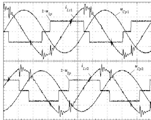
Figure 6: Measured voltages and currents of resonant converter
