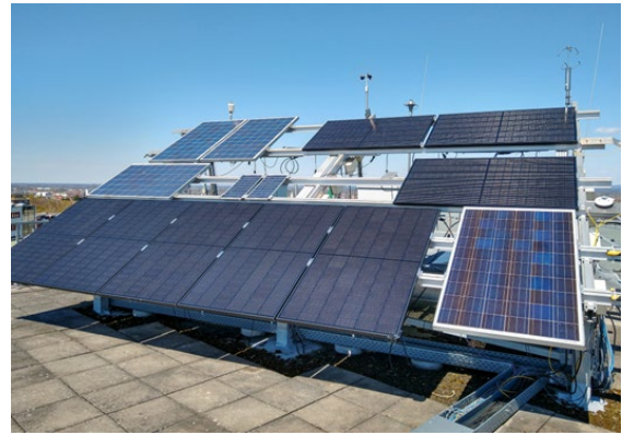
Figure 6: Configuration of PV modules of PV outdoor laboratory for electrical energy yield comparison of microinverters using eight equal, calibrated PV modules (of 360 W_p each) as inputs.
