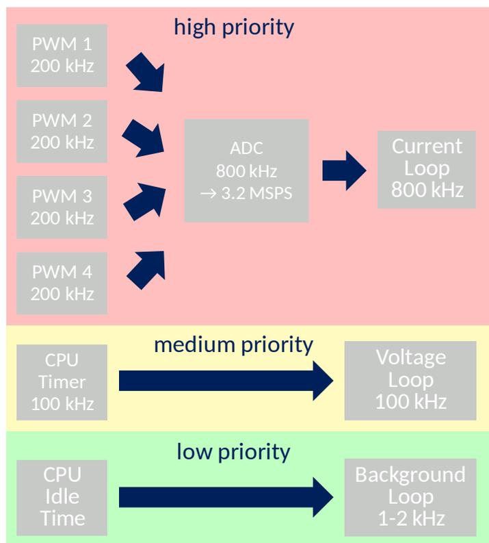
Figure 7.1: There are three different loop function priority levels with distinct execution rates.
