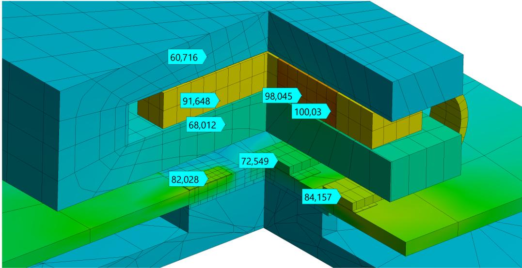
Figure 5.4: Cutting plane - temperature distribution of the magnetic component
