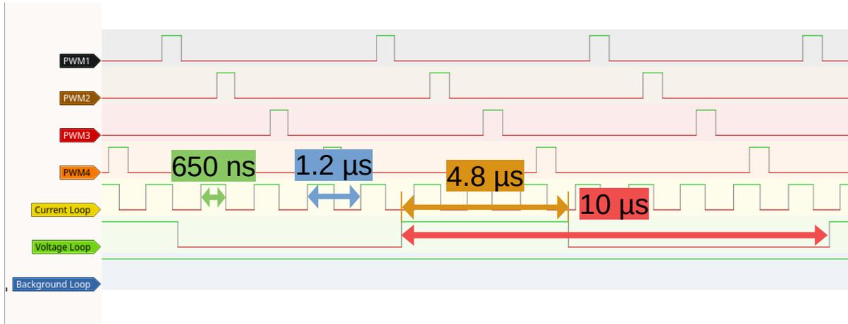
Figure 7.2: Capture of the execution times (green and orange marked) and execution period (blue and red marked) of the current loop and the voltage loop.
