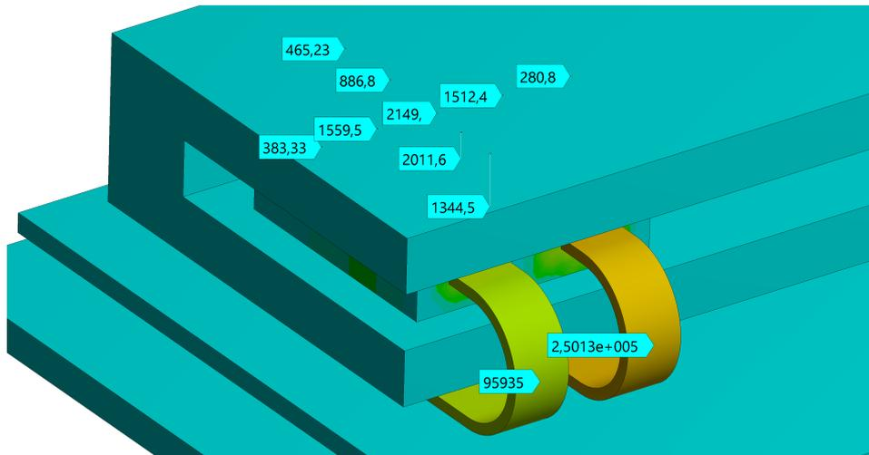
Figure 5.5: Heat flux densities in  $W/m^2$  of the windings and the ferrite yoke
