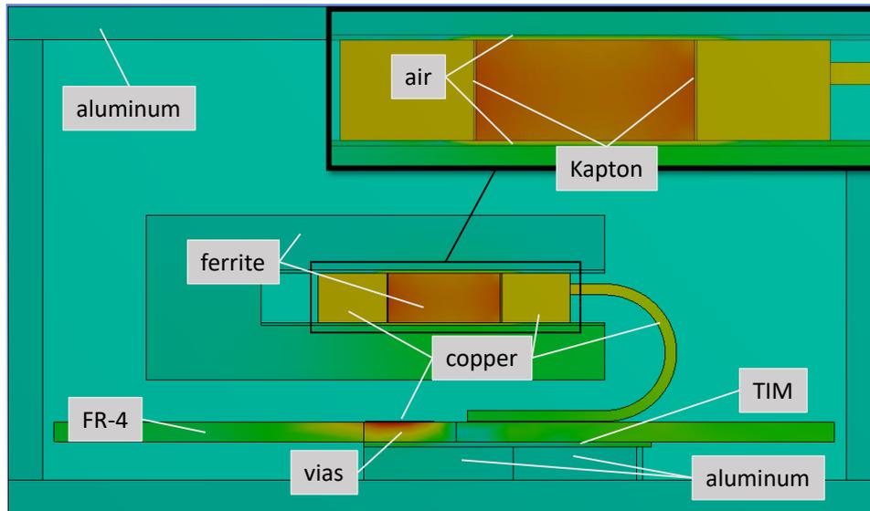
Figure 5.1: Material assignments to the simplified CAD model
