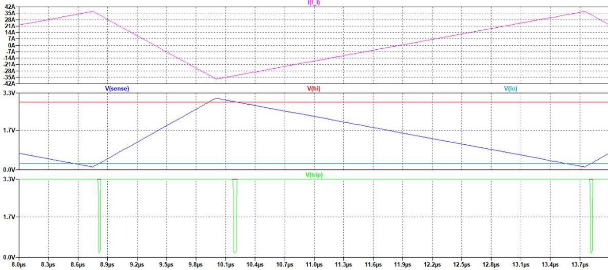
Figure 6.2: Results of the LTSpice simulation of a window comparator using the LMV339 and current limits of  $\pm 33\text{A}$ .
