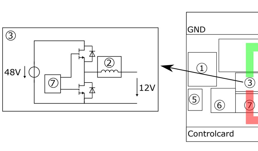
Figure 4.2: Schematic structure of the half-bridge.
