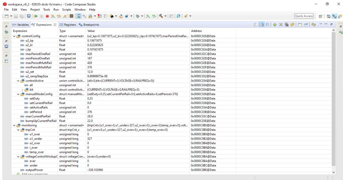
Figure 7.4: Screenshot of the IDE Code Composer Studio showing the variable watches used to control the converter during operation.
