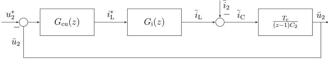
Figure 8.2: Voltage control loop based on [8] but with a correction on the capacitor's transfer function.
