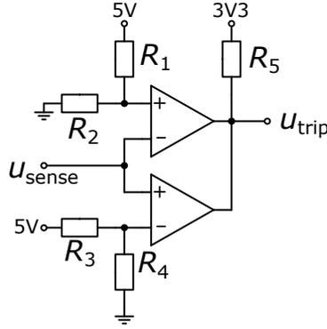
Figure 6.1: Chosen implementation of the window comparator circuit.
