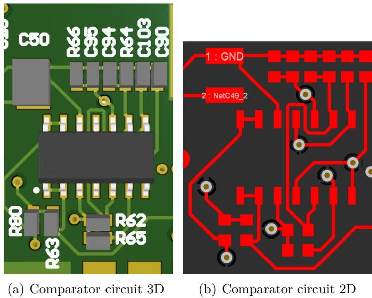
Figure 4.7: Comparator circuit
