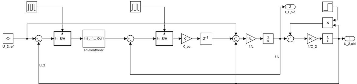
Figure 8.3: Simulink model for the control of one rail.
