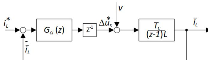
Figure 8.1: Current control loop [8].
