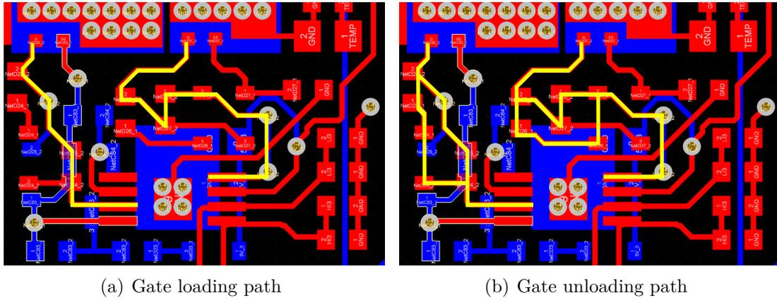
Figure 4.6: PCB layout of the driver circuit
