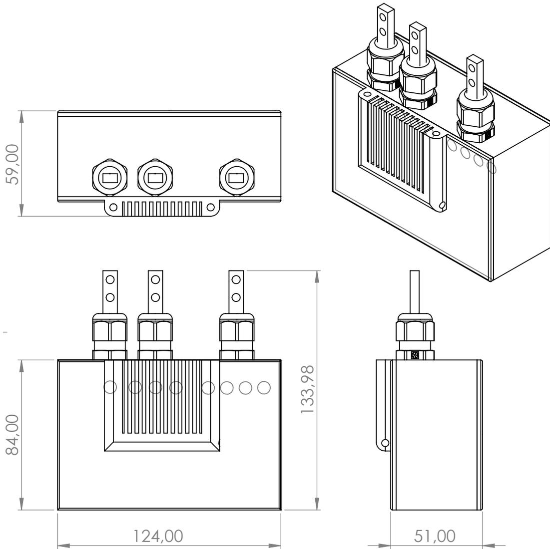
Figure 3.1: Housing with all components.
