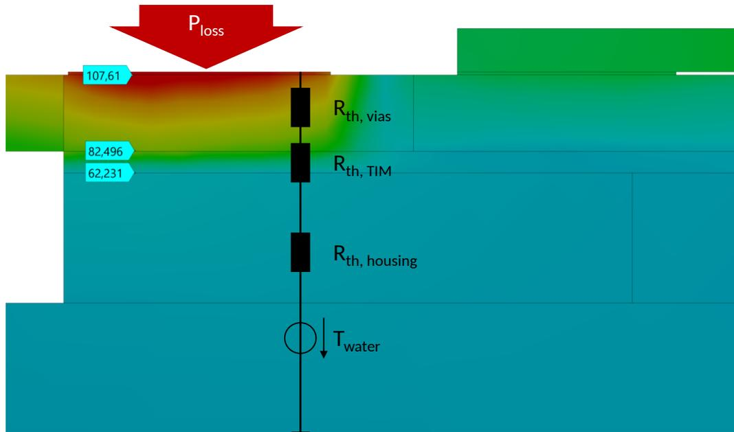
Figure 5.2: Cutting plane - temperature distribution in °C of low-side GaN - Thermal equivalent circuit
