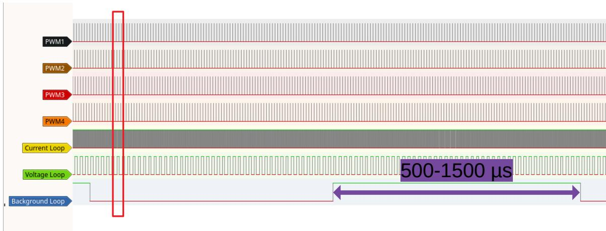
Figure 7.3: Capture of the execution time of the background loop (marked violet). The value is not fixed and depends on the CPU time used by the other loop functions as well as the use of the RFO. The red box corresponds to the time period shown in figure 7.2.
