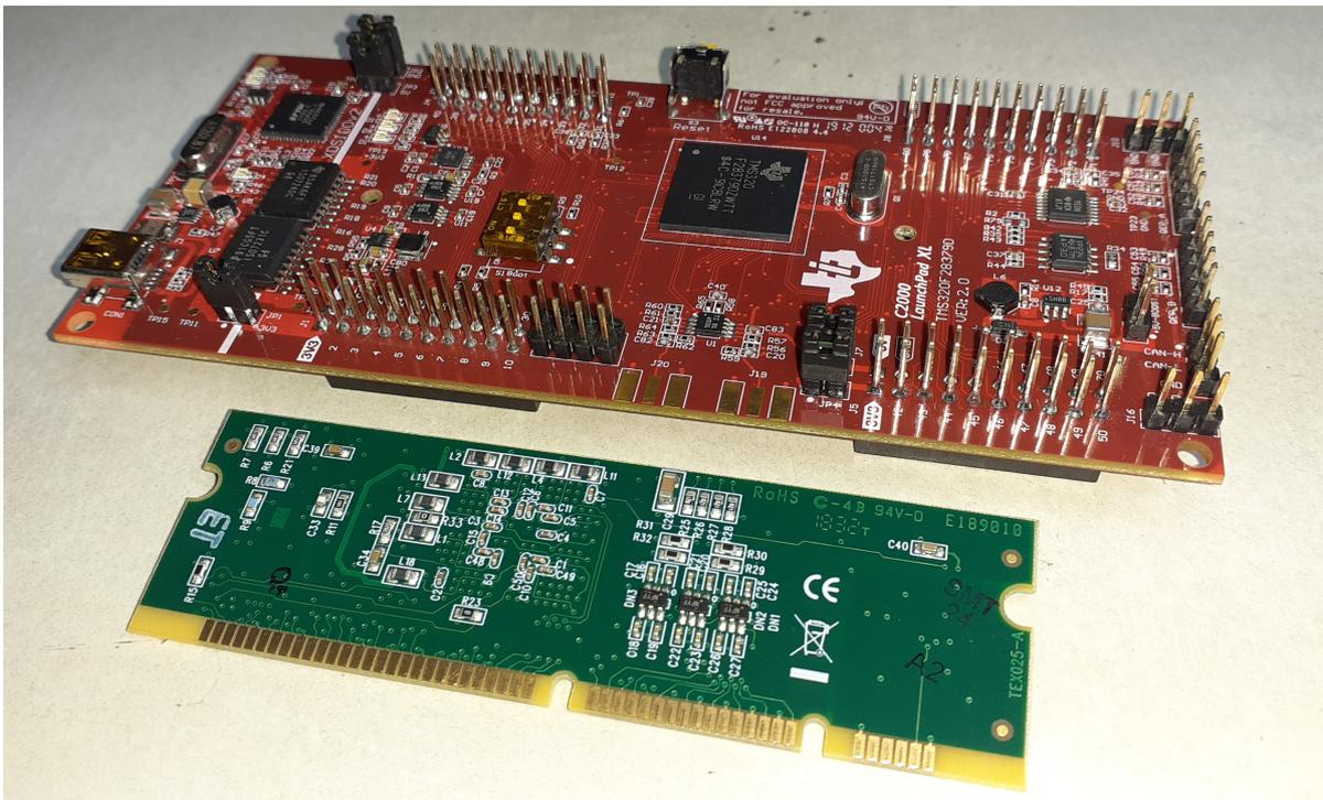
Figure 2.1: A F28335 control card (in front, green) next to the F28379D-Launchpad (red).
