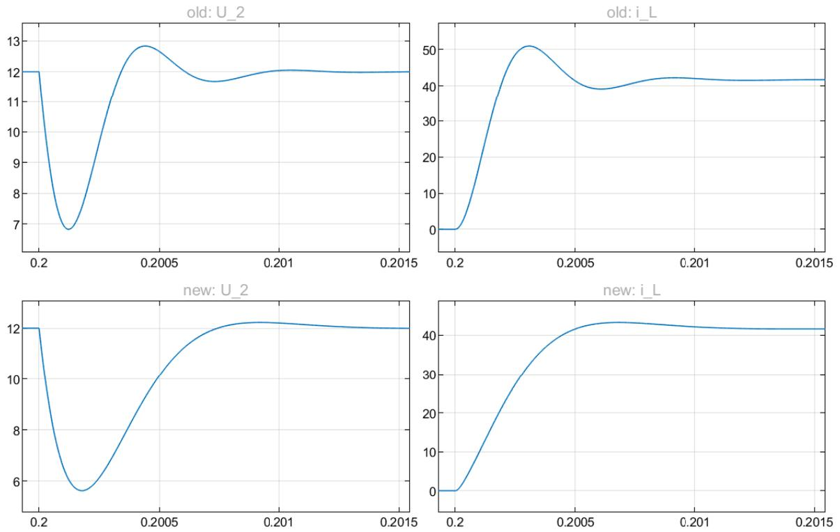
Figure 8.4: Results of the Simulink simulation comparing the old and new control's behavior when applying a load jump of 500 W.
