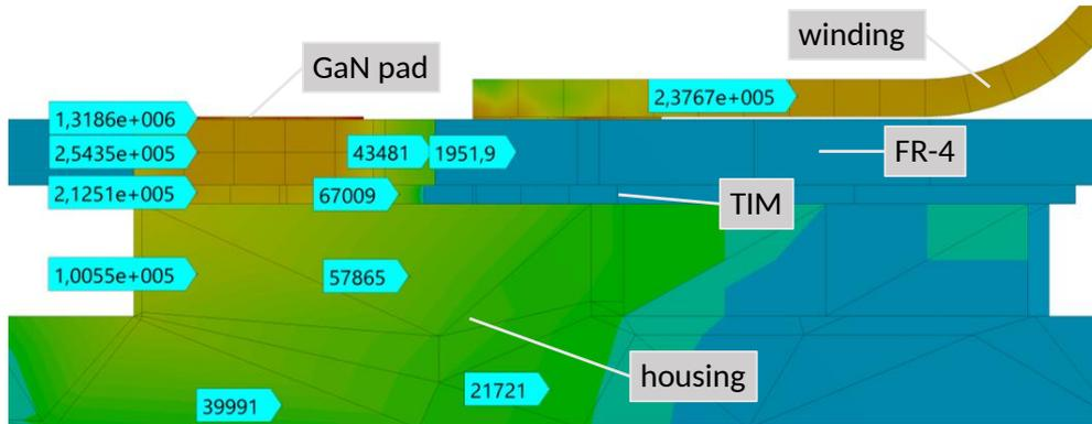
Figure 5.3: Heat flux densities in  $\text{W}/\text{m}^2$  - Plane cut of a low-side GaN
