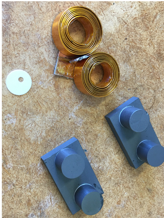
Figure 5.3.: The basic inductor components: winding, air gap material and ferrite core
