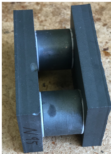
Figure 5.7.: The white air gap material is visible at the surface between the cuboid and the cylinder
