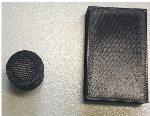
Figure 5.1.: 3D-Print from the cuboid and cylinder as a model of the ferrite parts
