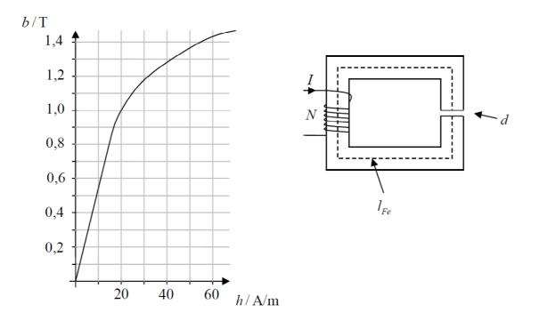
The flux density in the iron core B = 1.0 T.
