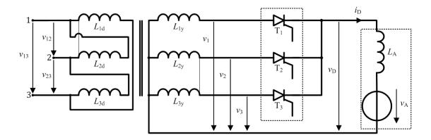
Figure 1: Three-phase half-wave controlled rectifier
