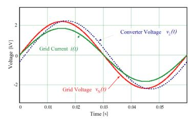
Figure 2: Voltages and currents transformed to the secondary side of the transformer
