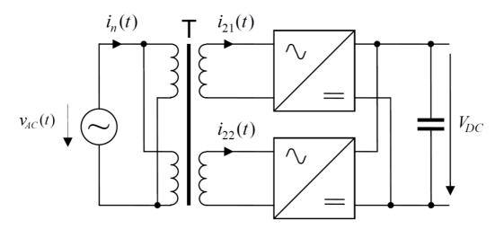
Figure 3: Power supply for an electric locomotive
