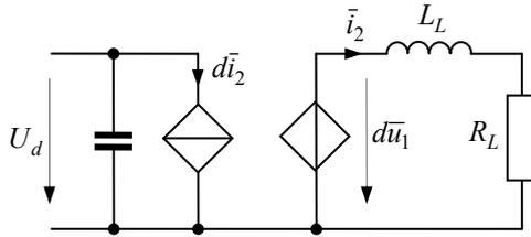
**Fig. 6** Equivalent circuit of averaged buck converter model
