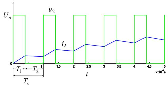
**Fig. 2** Voltage and current of buck converter
