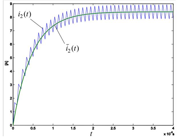
**Fig. 7** Simulation of averaged model vs. switched mode-simulation
