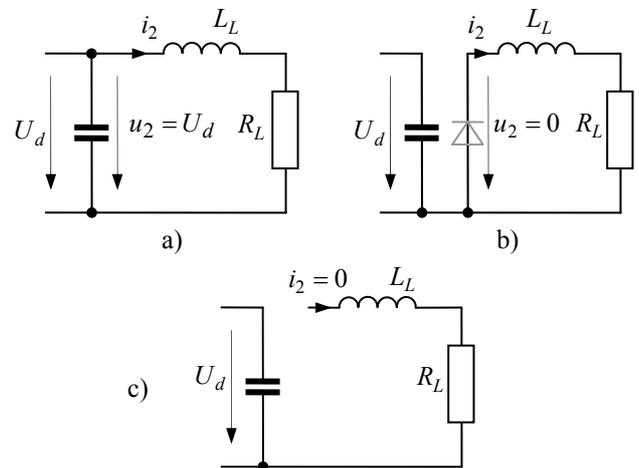
**Fig. 4** Equivalent circuits of buck converter
