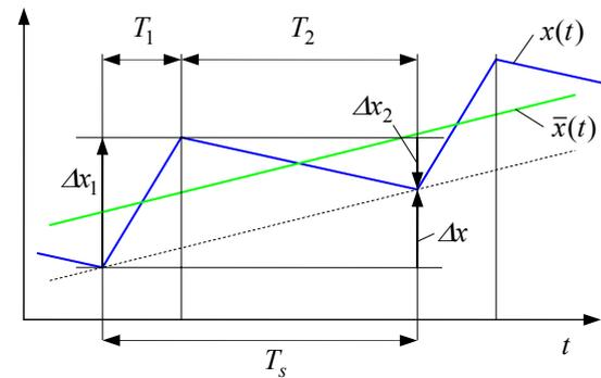
Fig. 5 State variable during a switching period
