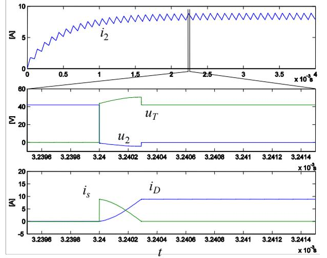
**Fig. 9** Voltages and currents transients during switch-off of the transistor
