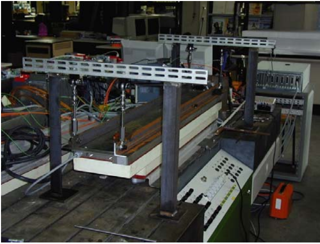
Fig. 7: Test bed for measurement of thrust and normal force
