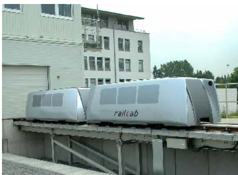
Fig. 2: Linear motor driven test vehicles
