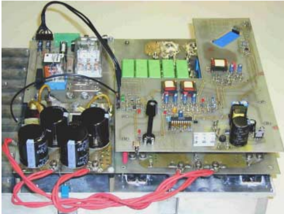
Fig. 16 Prototype of a 140A/4kW Welding Power Supply (left: input filter and rectifier, right: DC-DC Converter)
