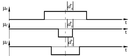
Fig. 4 Symmetrical pulse pattern without zero component
