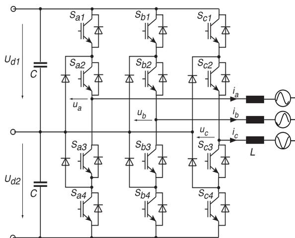
Fig. 1 Basic circuit of three-level PWM converter
