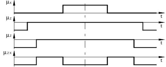
Fig. 7 Final symmetrical pulse pattern for low THD
