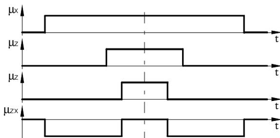
Fig. 8 Pulse pattern for low voltage level
