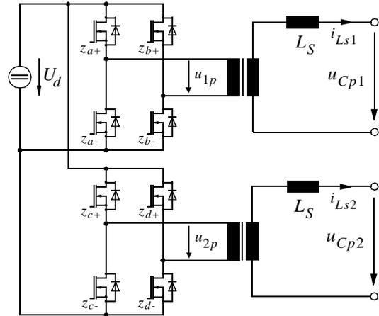
Figure 4: Two-phase resonant converter
