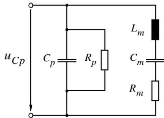
Figure 2: Equivalent circuit of USM
