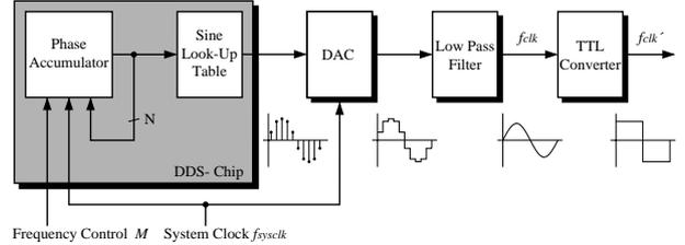
Figure 11: Direct Digital Synthesizer
