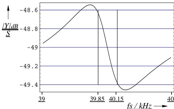
Figure 3: Admittance curve of network in Fig. 1
