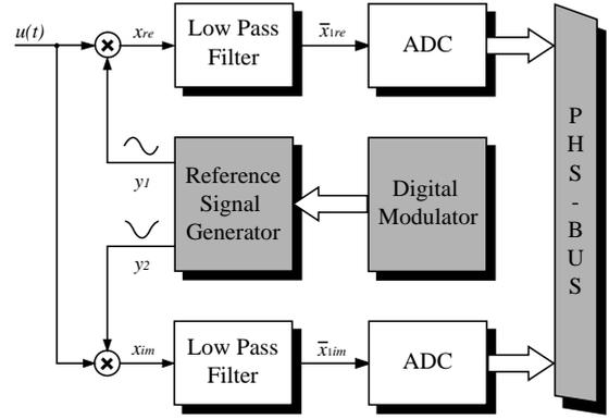
Figure 13: Measuring system by analog demodulation
