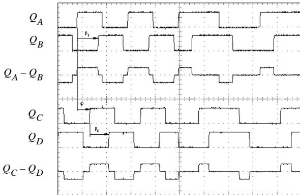
Figure 12: Measured output signals of digital modulator
