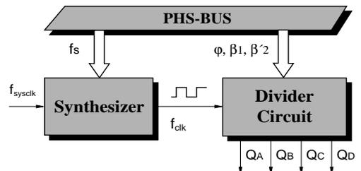
Figure 9: Basic concept for the digital modulator
