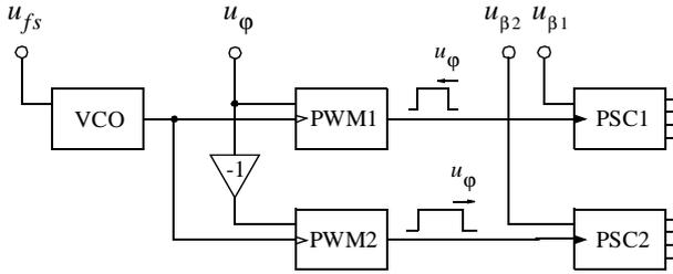
Figure 7: Analog control circuit for two-phase resonant converter
