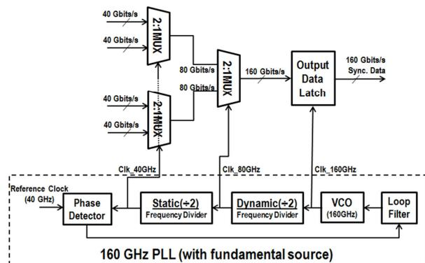
Fig. 1. The proposed 160 Gbits/s 4:1 MUX architecture
